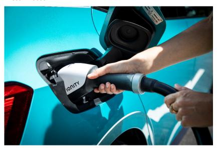
IONITY is one of the first charging network operators in Europe to offer Plug & Charge technology. With Plug & Charge, the car automatically authenticates itself to the charging station and carries out the charging and payment process.
